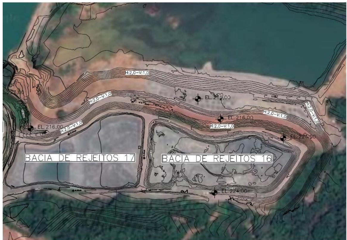
Figure 18-4: Active Tailings Dams 16-17
